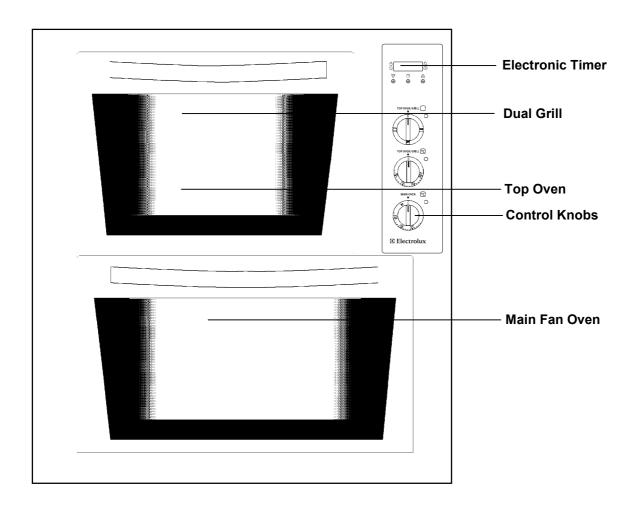
Your built-under appliance comprises of a conventional oven and dual grill in the top compartment. The top oven is convenient and economical for mid-week use because of its size.
